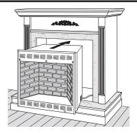
Figure 20 - Inserting Firebox Into Cabinet Mantel
